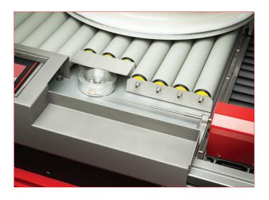
THE WHEEL INSPECTION SEQUENCE: The VEESCAN is designed to lift the wheel and fix it with an automatic adaptor that uses the wheel inertia to center it. The VEESCAN offers an integrated roller tray for easy maneuverability and integration into a conveyor system and also features an automatic hub size adaptor. The VEESCAN can test wheels up to 900mm (35") diameter.
