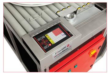
**GREAT EDDY CURRENT TECHNOLOGY:** The VEESCAN works in conjunction with the ETHER NDE AEROCHECK+ eddy current flaw detector. The flaw detector sits behind a protective tough polycarbonate window and provides the unit with the eddy current technology for the inspection.
