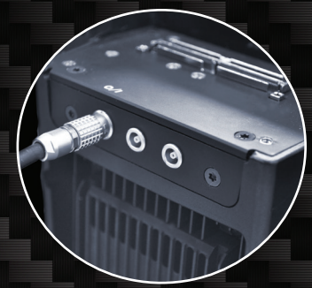
IPEX PAUT connector, 2 pulser-receivers and Encoders (I/Os)
