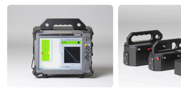
The new PECT instrument comprises a ruggedized tablet computer connected to a data acquisition unit.
