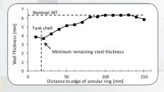
The above graph represents an example result of an annular ring inspection with the MAXWELL PECT, showing severe wall loss close to the tank shell. The corroded area extends over a length of about 80mm (3.15ins) in this case.
