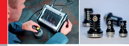
We offer our precise ultrasonic probes with different frequencies and transducer sizes. Choose the most suitable probe for your application, depending on material characteristics, thickness and geometry of the work piece.
