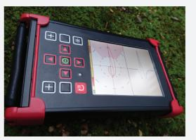
Area of Inspection: Horizontal Stabilisers **Probe: High & Low Frequency**
